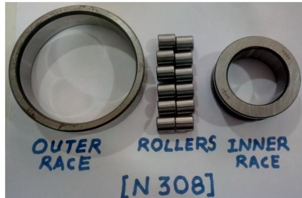
Figura 1: N308 Bearing Parts
