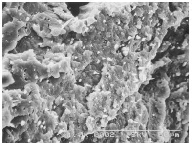
Figure 4: SEM image of PET/5.0%LCP blends with PMDA reactive additive. Good adhering and plastically deforming LCP fillers
