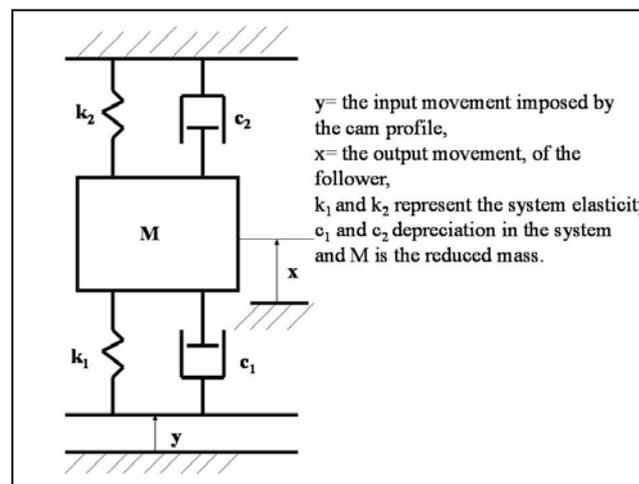
Figure 1: Dynamic model with a degree of freedom with double internal damping
