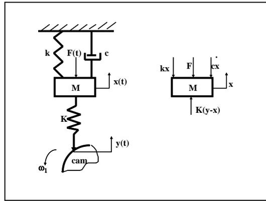
Figure 13: Mono - dynamic model, with internal depreciation of the variable system
