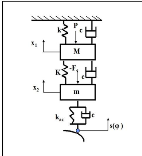
Figure 8: Dynamic damped two-mass model
