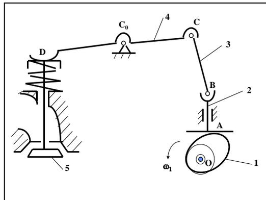
Figure 12: The kinematic scheme of the classic model, with distribution mechanism
