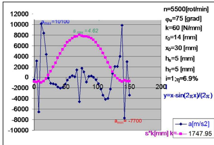
Figure 14: Dynamic analysis using the A3 dynamic model
