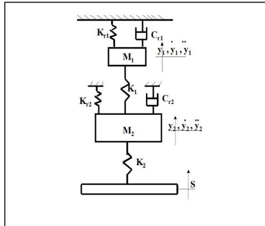
Figure 5: Dynamic two-degree, dual damping model
