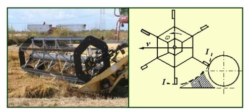
Graph 3: Computer model of harvester reel movement
