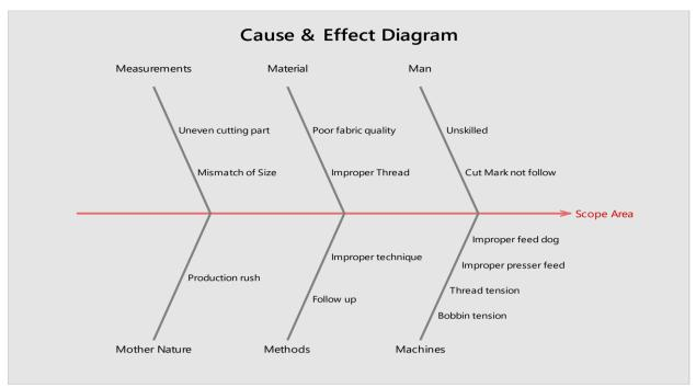
Figure 2: Cause and effect diagram for scope area.
