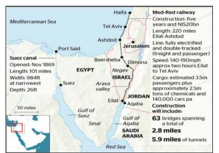
Figure 5: The Red-Med railway as an alternative to the Suez Canal
