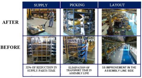
Figure 13: Improvements implemented in Assembly Line
