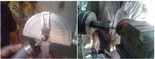
Figure 2: Alteration of drill tool geometry using Tool and Cutter grinder
