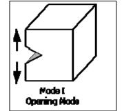
Figure 3: Mode I Fracture Modes
