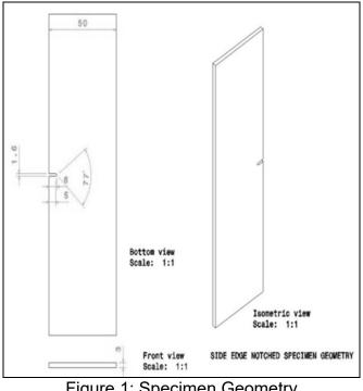
Figure 1: Specimen Geometry
