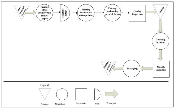
Figure 8: Invoice manufacturing process
