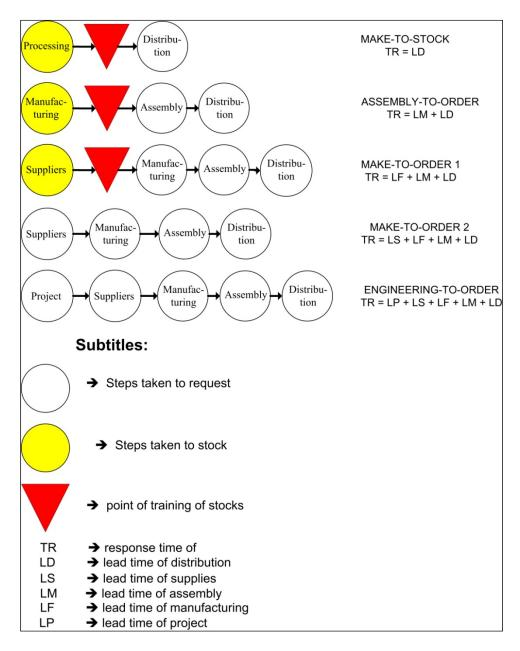
Figure 1: The ways of responding to the demand of production systems Source: Godinho Filho (2004).
