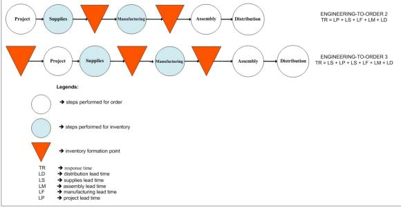
Figure 9: Company's Engineering-To-Order process flow
