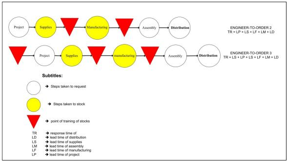
Figure 11: Process flow of Engineering-To-Order company's
