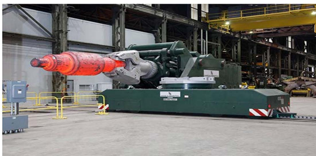
Figure 12: Forging Manipulator (Rail Mobile)
