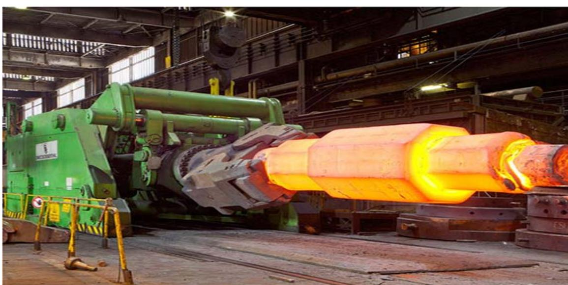
**Figure 6: Forging Manipulator (Rail Mobile)**
