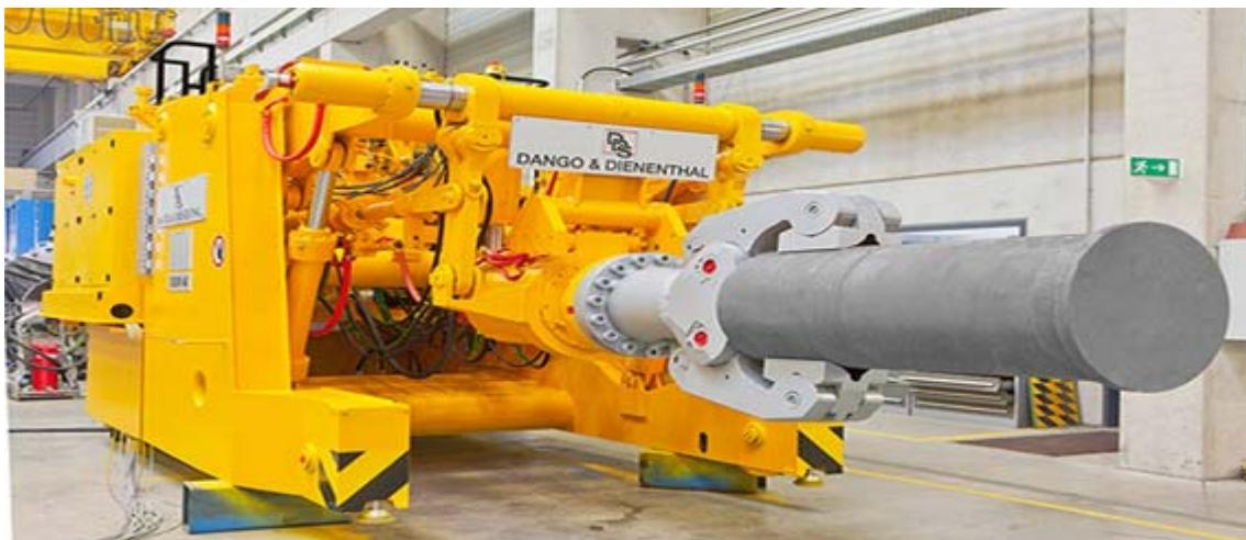
**Figure 5: Forging Manipulator (Mobile)**
