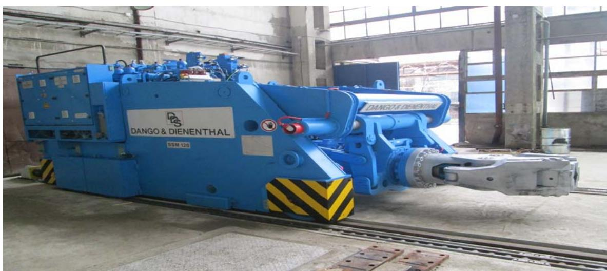
Figure 13: Forging Manipulator (Rail Mobile)
