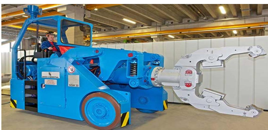
Figure 9: Forging Manipulator (Independent Mobile)
