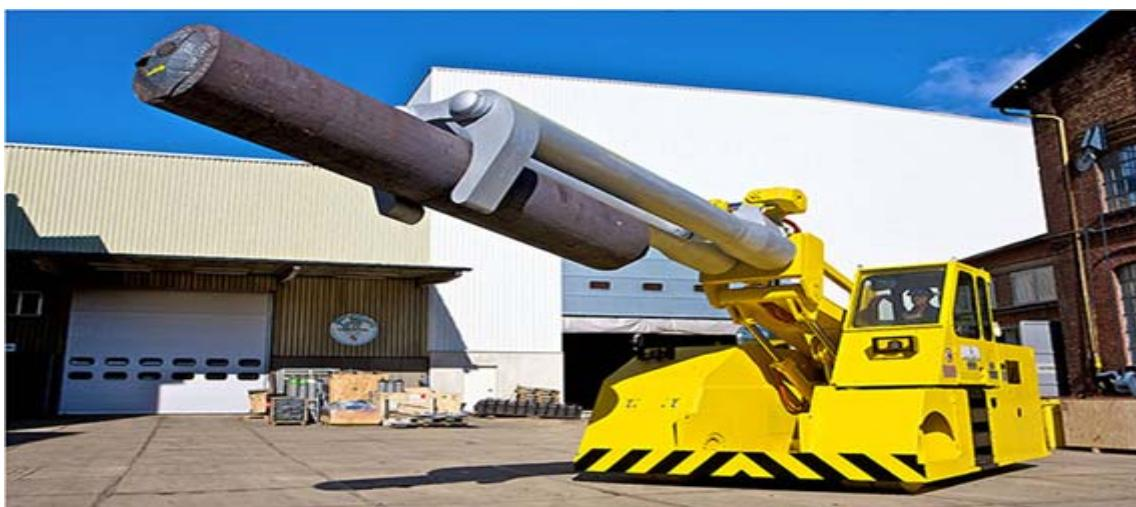
Figure 11: Forging Manipulator (Independent Mobile)
