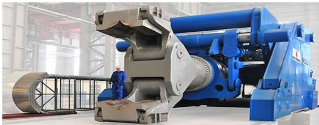
Figure 1: Forging Manipulator (Rail Mobile)
