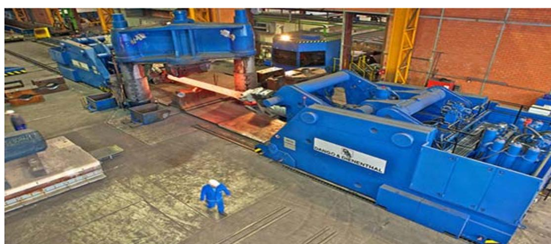
Figure 3: Forging Manipulator (Rail Mobile)
