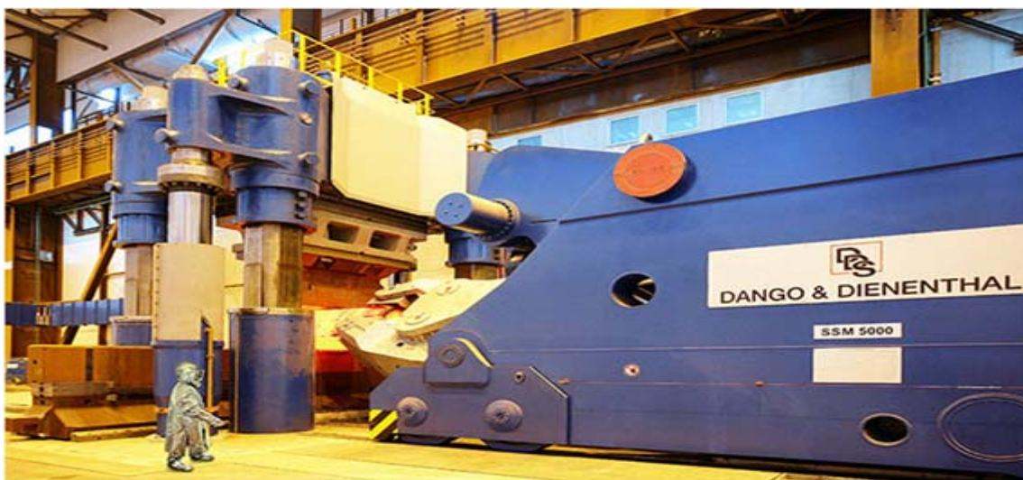
**Figure 4: Forging Manipulator (Rail Mobile)**
