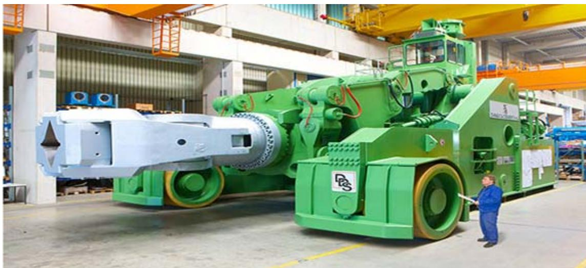
Figure 7: Forging Manipulator (Independent Mobile)
