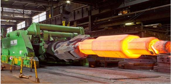
Figure 6: Forging Manipulator (Rail Mobile) Source: Dango & Dienenthal
