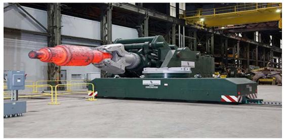
Figure 12: Forging Manipulator (Rail Mobile) Source: Dango & Dienenthal
