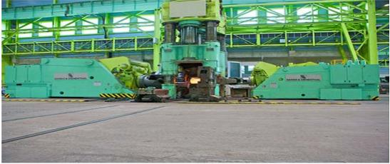
Figure 2: Forging Manipulator (Rail Mobile) Source: Dango & Dienenthal
