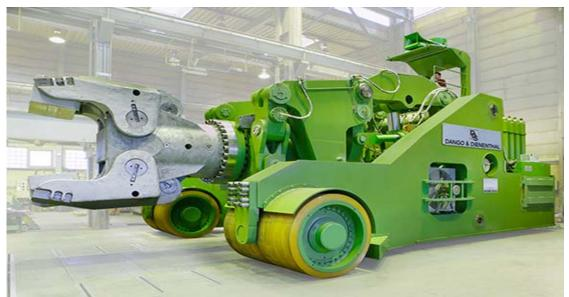
Figure 8: Forging Manipulator (Independent Mobile) Source: Dango & Dienenthal
