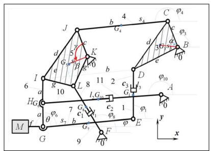
Figure 16: General cinematic schema of a forging manipulator main mechanism
