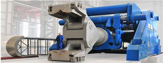
Figure 1: Forging Manipulator (Rail Mobile) Source: Dango & Dienenthal
