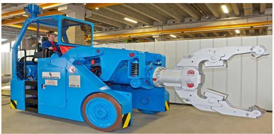
Figure 9: Forging Manipulator (Independent Mobile) Source: Dango & Dienenthal
