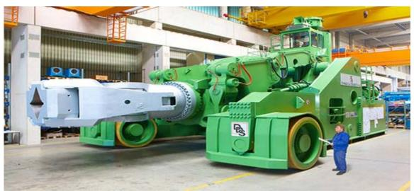
Figure 7: Forging Manipulator (Independent Mobile) Source: Dango & Dienenthal
