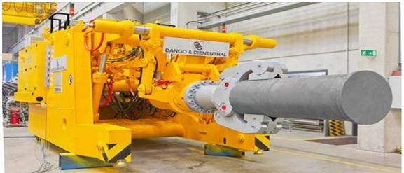
Figure 5: Forging Manipulator (Mobile) Source: Dango & Dienenthal
