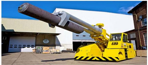
Figure 11: Forging Manipulator (Independent Mobile) Source: Dango & Dienenthal
