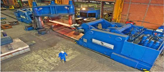
Figure 3: Forging Manipulator (Rail Mobile) Source: Dango & Dienenthal
