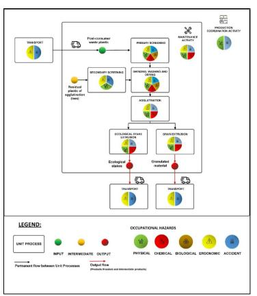
Figure 1: Fluxogram of the process and identification of occupational hazards.
